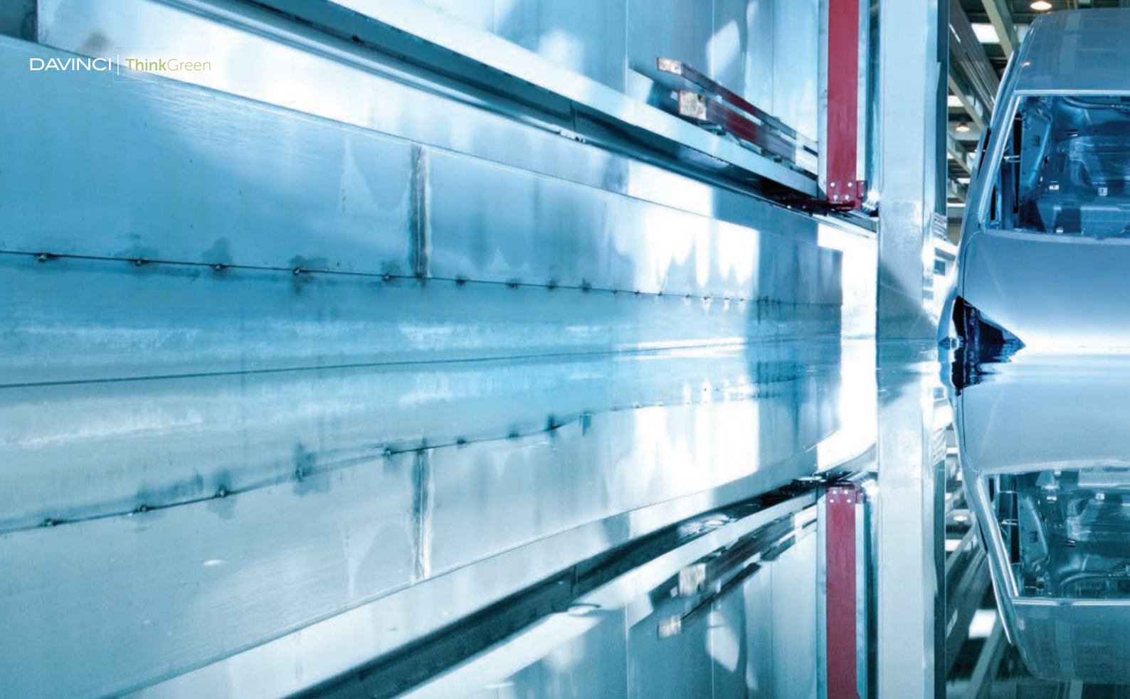
The flexible E-Shuttle dip coating conveyor minimizes carry-over.
